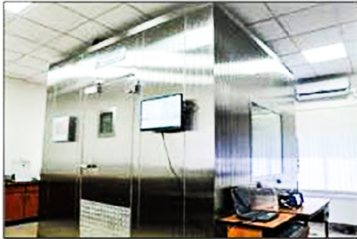
Fig 3: Walk in Type 222 Rn Calibration Chamber
