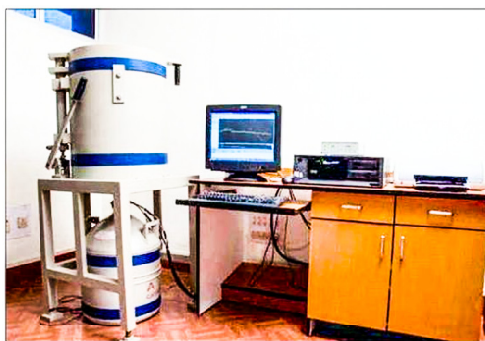
Fig 2: A View of HPGe Spectrometer Used in Present Study
